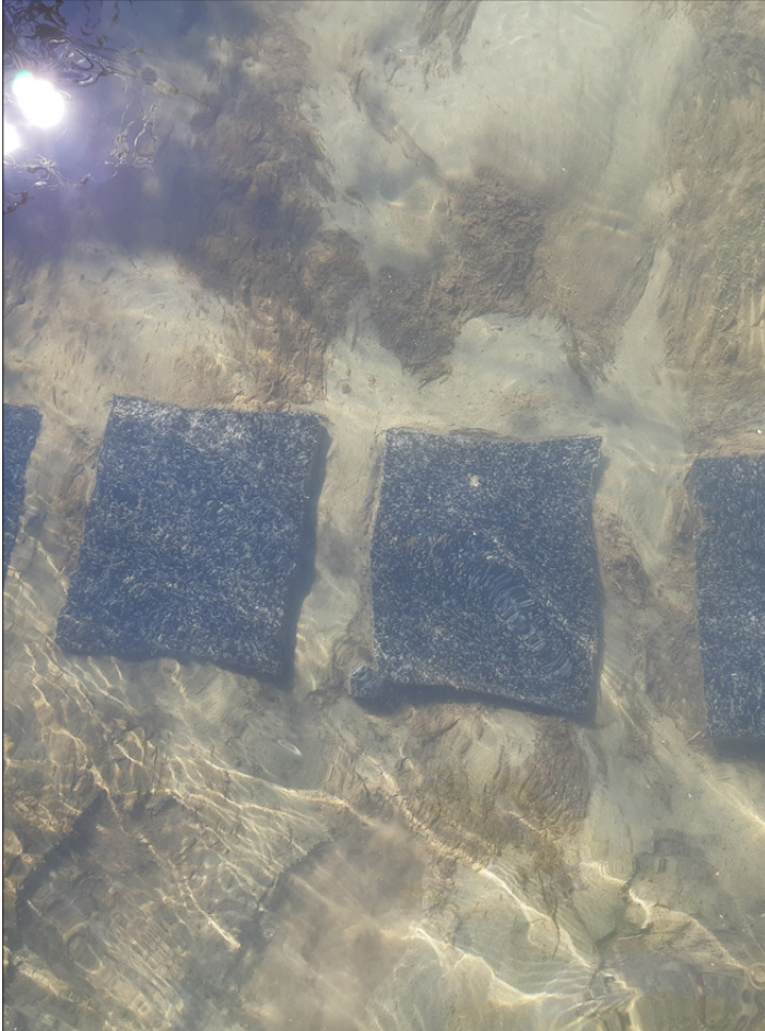
Figure 6. Flood (suspended sediment) collectors and bed load sediment tiles
