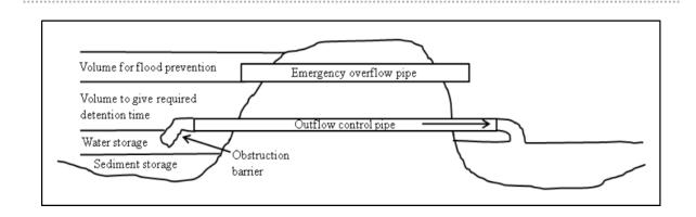
Figure 25: Generic schematic section of a peak runoff control structure
