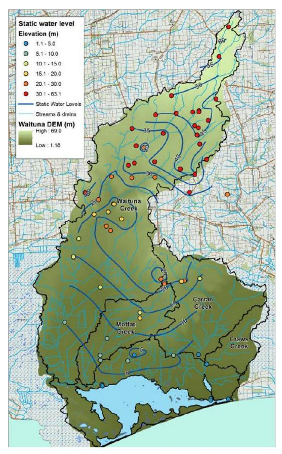
Figure 11: Static water levels from a survey carried out by Environment Southland in 2012 (Rekker and Wilson, 2016)
