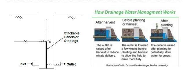
Figure 26: Schematic of how controlled drainage (or drainage water management) works
