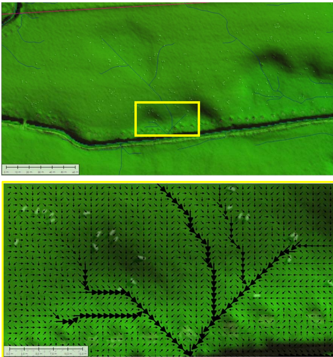
Figure 5.10: Flow direction and convergence at the paddock scale. The top image shows the riverlines generated in Section 5.4. The bottom image illustrates flow convergence with 1 arrow for every 1m 2 .
